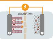
A porous separator keeps the battery electrodes apart. Charging the battery for long periods or inflicting a mechanical blow can damage the separator, causing the battery to discharge rapidly and generate a lot of heat
