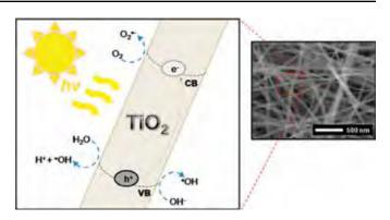
composition were synthesized by electrospinning to optimize photocatalytic treatment efficiency. Nanofibers of controlled
