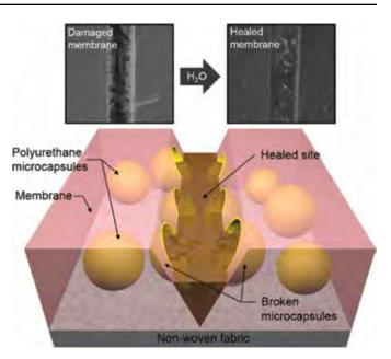
original membrane's performance, respectively. The results of this study show that microcapsule-embedded membranes are a promising approach to fabricating versatile, next-generation membranes that can self-heal.
