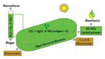
biomass content remained constant at  $49 \pm 2\%$ ,  $9 \pm 0\%$ , and  $1 \pm 0\%$ , respectively, over the 175 days of experimentation. The high carbohydrate contents (60–76%), inversely correlated to biogas flow rates, would allow the production of ~100 L of ethanol per 1000 m<sup>3</sup> of biogas upgraded under a biorefinery process approach.
