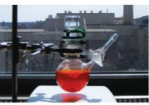
SUNLIT SYNTHESIS Visible light helps Ru(bipy)<sub>3</sub>Cl<sub>2</sub> catalyze [2+2] enone cycloadditions.
