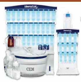
**NUKE IT** CEM's automated microwave peptide synthesizer reduces solvent use and reaction times.
