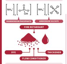
Other ingredients include gum-based thickeners, which hold the cloud of retardant together as it's applied from the air. Flow conditioners allow the powder to be easily transferred and mixed. The red color of Phos-Chek. which aids air crews in applying it, derives from iron(III) oxide or a nonpermanent, light-sensitive dye.
